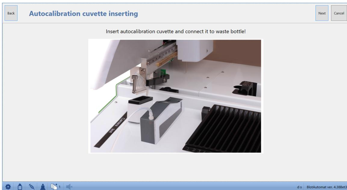
The user places the calibration cuvette on the upper case of the instrument according to the picture and connects the cuvette tube to the waste bottle with a self-closing clutch.
