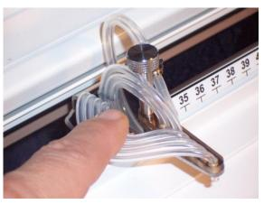
The tubec ,C,D,G are inserted in front of the arm pivot, A,B,E,F behind it.
