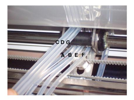
Secure the tubing by means of the plastic wrap to the dispensing arm body. Tight wrap carefully not to press dispense tubing.
