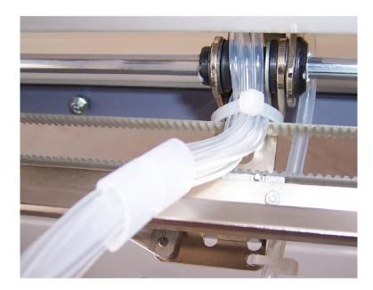
Poke the tubes through holes above the pumps and connect them to the tube-to-tube connectors of the rihgt pump tubes. The left pump tube is the input, the right tube is the output.
